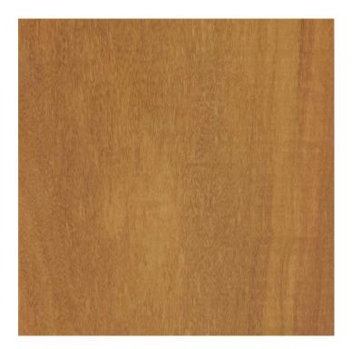
Garapa is a light yellow to honey-brown colour and its interlocked grain has a fine texture. It is a very durable timber that resists rot, decay and fire.
